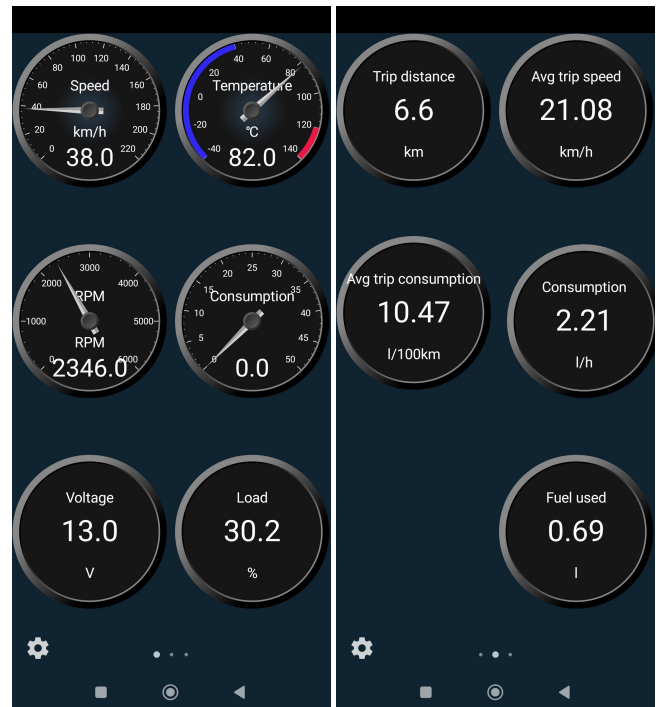
Fig. 3. Some sensors and parameters can be read using OBD Mary.
